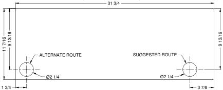
The holes shown are the best locations to route the refrigerant lines, condensate drain, and electric. For installations where the line set will be accessible on the backside of the wall, use the suggested route. When that is not possible, and the line set will be run inside the wall before the drywall is installed, use the alternate route. This will leave the flare connections exposed so they can be connected after the walls are finished.
