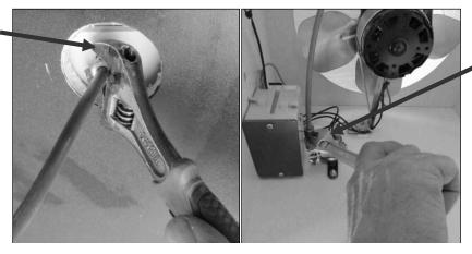
Wrench inside to keep solenoid valve from spinning
