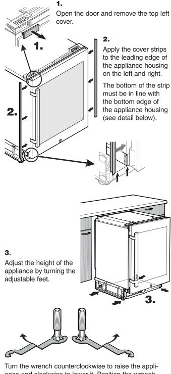
ance and clockwise to lower it. Position the wrench accordingly.
