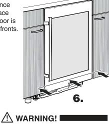
When sliding in the appliance, make sure not to damage the power cord!
