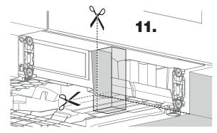
**IMPORTANT** If the foam block is not installed, the appliance will not deliver optimal refrigeration performance during operation.
