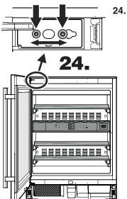
24. Undo screws and slide hinge bracket to the right or left. Tighten screws.
