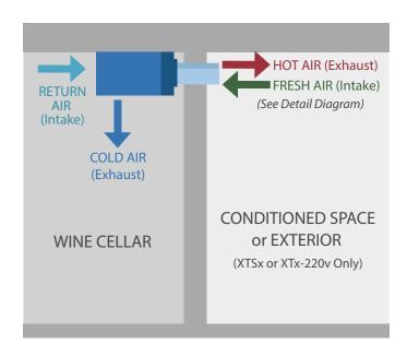
\* The hot air exhaust can be rear or top vented.
