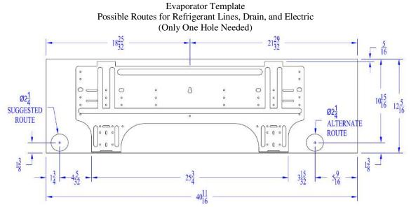
The holes shown are the best locations to route the refrigerant lines, condensate drain, and electric. For installations where the line set will be accessible on the backside of the wall, use the alternate route. When the line set will be run inside the wall before the drywall is installed, use the suggested route. This will leave the flare connections exposed so they can be connected after the walls are finished.
