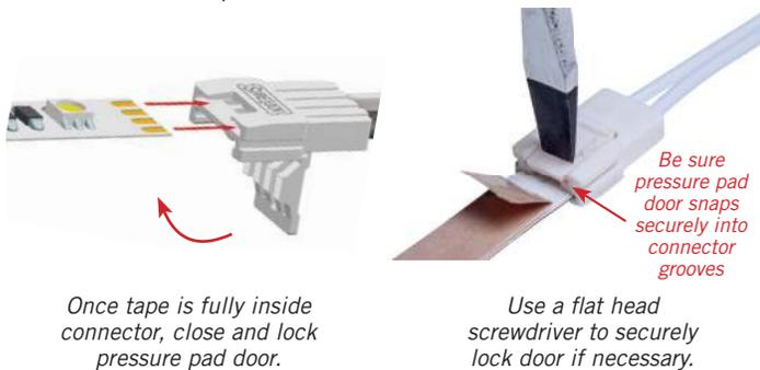
Once tape is fully inside connector, close and lock pressure pad door.
