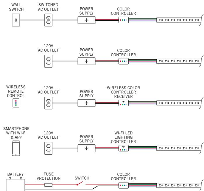
Interior RV and boat applications can be powered directly by a battery. Make sure the LED tape lighting that you are using matches the voltage of your RV or boat.
