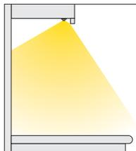
**If your countertop is reflective**, install the LED tape lighting on the inside back of the cabinet lip frame with the LEDs facing towards your backsplash. This method helps eliminate unwanted light reflections and bright spots reflecting off your countertop. Because of the wide beam angle of the tape light, this mounting position will still provide ample lighting.
