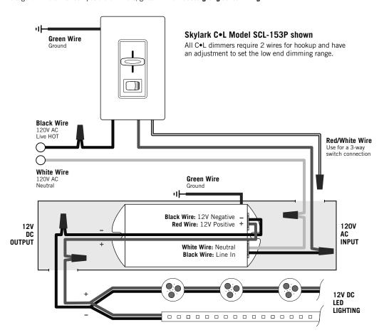
Power supply is for direct wire only and includes NEMA 1 listed metal enclosure with eight (8) 7/8" knockouts. After removing knockouts, install suitable strain reliefs and route wires appropriately to fit installation location.
