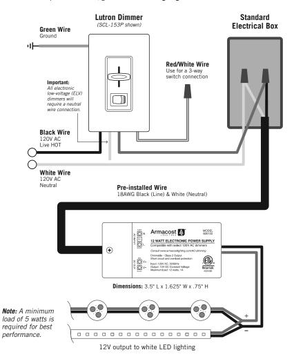
Power supply is for direct wire only. All wiring must be in accordance with national and local electrical codes, low voltage Class 2 circuit. If you are unclear as to how to install and wire this product, contact a qualified professional.
