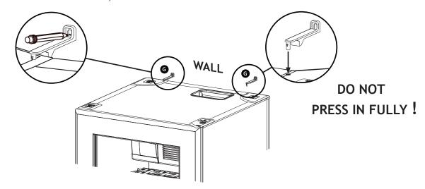
DRILL USING 1/4" (6 - 6.5 mm) DRILL BIT AND TAP IN ANCHORS
