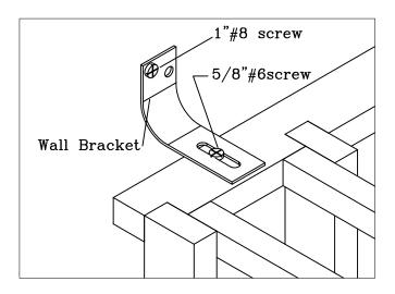
Secure rack to wall by attaching wall brackets to top back spacer bar. You will have 1 bracket on the left and 1 on the right.
