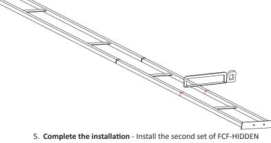
following the procedure in step 3 and refer to the Floor to Ceiling Frame (FCF) installation instructions to complete the remaining installation steps, ensuring that screws are securely fastened into both mounting holes in each FCF-HIDDEN bracket.
