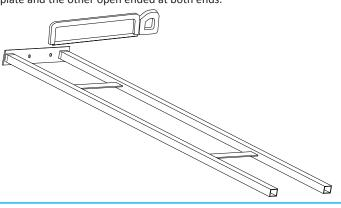
3. Insert the FCF-HB pieces - Slide the FCF-HIDDEN pieces into the open ends of the Floor to Ceiling Frame, with the mounting holes positioned toward the front and back of the Frame as shown below. For maximum rigidity when installed, it is recommended that a self drilling screw be inserted through the side wall of the frame and into the "U" channel of each bracket.
